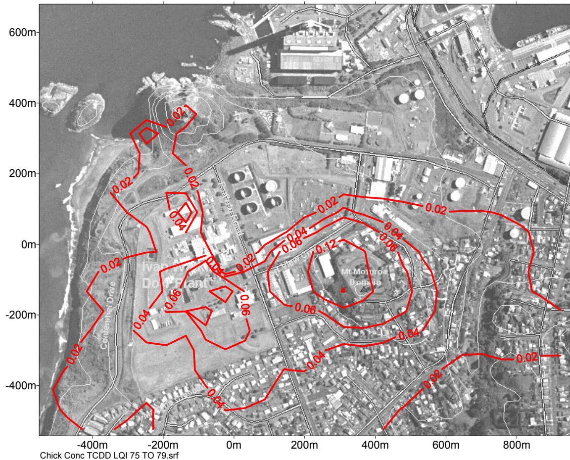
Figure 6. Predicted incremental 2378-TCDD chicken meat concentrations (ng-TEQ/kg-FW) from emissions from the IWD liquid waste incinerator between 1975 and 1979
