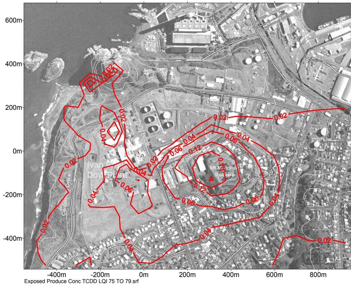
Figure 7. Predicted incremental 2378-TCDD exposed above-ground produce concentrations (ng-TEQ/kg-DW) from emissions from the IWD liquid waste incinerator between 1975 and 1979
