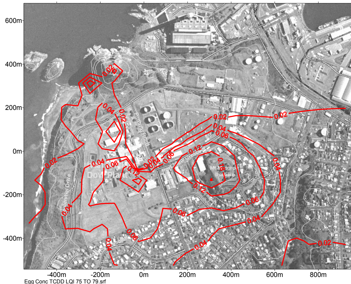
Figure 5. Predicted incremental 2378-TCDD egg concentrations (ng-TEQ/kg-FW) from emissions from the IWD liquid waste incinerator between 1975 and 1979
